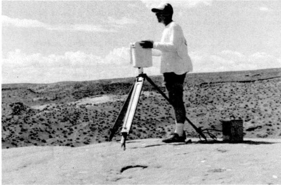
Figure 11. – Microwave receiver-transmitter at shore station. P801-D-81399
